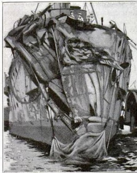
The Bow of the “Hawke,” the Damage being so Great That the Ram Has Been Mashed Flat
