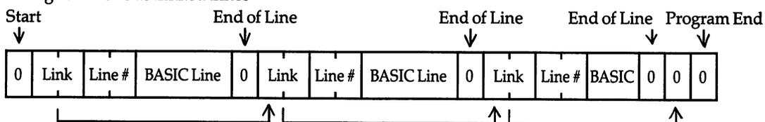
The built-in operating system automatically arranges BASIC as lines are typed in and entered (by pressing the RETURN key) at the keyboard. When you understand how lines are entered, you can modify BASIC to produce nonstandard effects. You could insert lines longer than usually possible, add normally unavailable line numbers, or arrange a line of BASIC to contain things it ordinarily couldn't.
