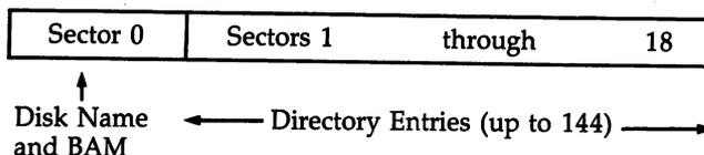
Each time a file is written, the BAM (Block Availability Map) is updated, so the system knows which sectors are free for subsequent recording. VIEW BAM on the demo disk prints a diagram of this map. To see how this works, load DISPLAY T&S and inspect track 18, sector 0. Its layout is described in Table 15-3.
