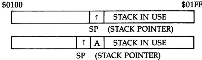
**Uses:** This instruction is used for temporary storage of bytes. It may be used to hold intermediate values of calculations produced during the parsing of numeric expressions, to temporarily store values for later recovery while A is used for other processing, for storage when swapping bytes, and for storage of A, X, and Y registers at the start of a subroutine.
