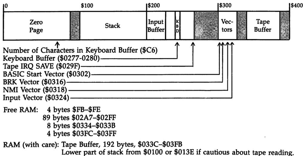
**BASIC warm start vector in (\$0302).** Normally \$A483, this can be directed either into the header or into the loaded program, perhaps spanning \$02A7-\$0303. Then ML LOAD and RUN will automatically run the BASIC program that comes afterward.
