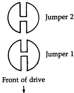
Cutting only jumper 1 changes the device number to 9. Cutting only jumper 2 changes it to 10. Cutting both jumpers changes it to 11. Note that opening the drive case to do this will probably void your warranty. *To avoid severe electrical shock, do not attempt any such operation until you have turned the drive off and unplugged every connector.* If you're not sure what's involved, get help from someone who understands electronics.
