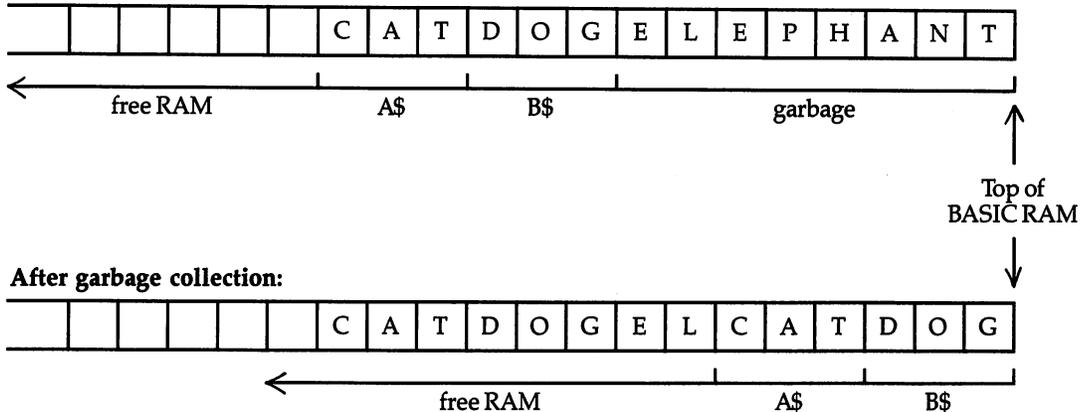
Let's suppose BASIC tries to set up a new string but finds there's insufficient room. It calls a routine, the same as FRE(0), to find out which of the strings after BASIC are still being used. Strings stored within BASIC itself are outside the scope of this algorithm and are ignored.
