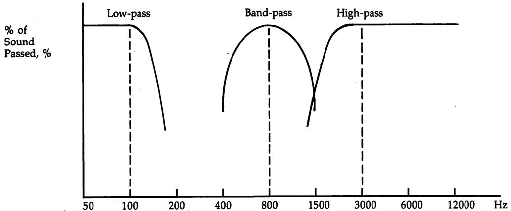
Low-pass filter with cut-off frequency 100 Hz
