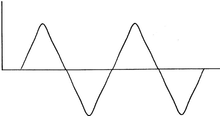
This is SID's closest approximation to a sine wave, and it sounds like a flute or xylophone. Four sinusoidal harmonics—the first, third, fifth, and seventh—add to form an approximately triangular waveshape.
