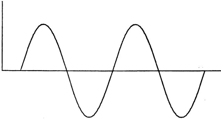
Circular motion generates sine curves; the SIN function describes this motion. As it happens, the prongs of a sounding tuning fork give a good approximation of sinusoidal motion. In fact, simple harmonic motion derives its name from the sound analogy.
