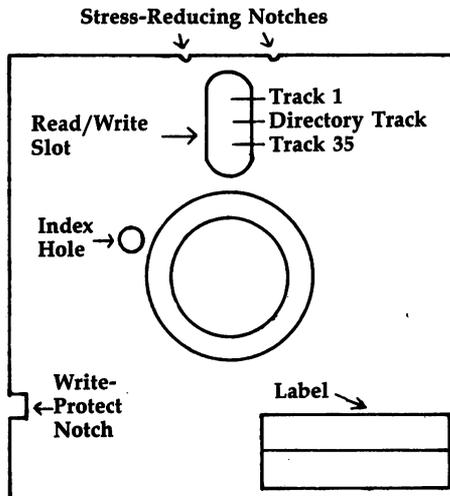
Diskettes are inserted label up, read/write slot foremost. Diskette labels are deliberately positioned away from the slot, to reduce the chance of fingerprint damage and to allow the label to be read when the diskette is in its dust cover. Writing on the label with a sharp implement—for instance, a ballpoint pen—may damage the diskette surface below. Always write on the label before putting it on the disk.
