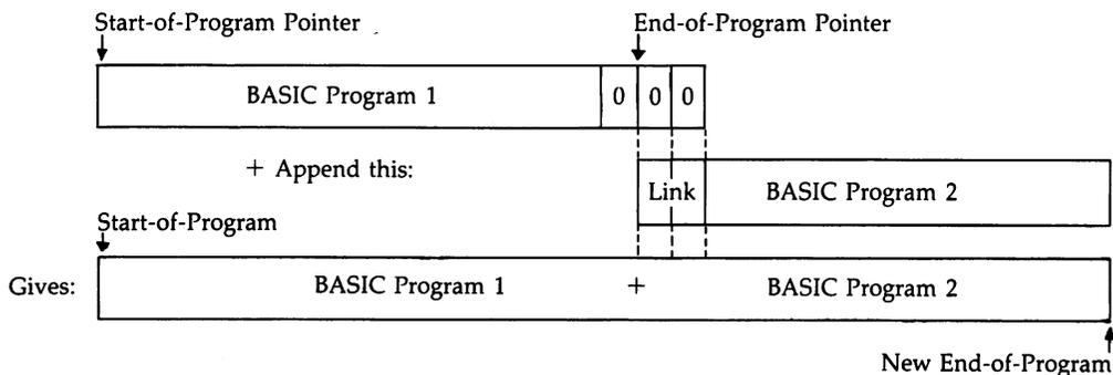
The easiest approach is to first enter `POKE 43, PEEK(45)-2:POKE 44, PEEK(46)` in direct mode; then load or type in the new lines of BASIC and `POKE 43,1:POKE 44,8` to start BASIC at \$800. Perfectly appended BASIC should be the result. Actually, this method is a shortcut; if `PEEK(45)` happens to be 0 or 1, you'll get an *ILLEGAL QUANTITY ERROR* and will need to edit your instructions to `POKE 43, PEEK(45)+256-2:POKE 44, PEEK(46)-1`, then continue as before.
