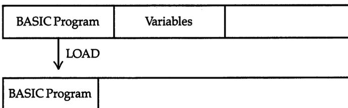
Note: LOAD command on first program causes new BASIC program to load, then run. In the diagram, the new program is shorter than the old, so variables' values are mostly retained.
