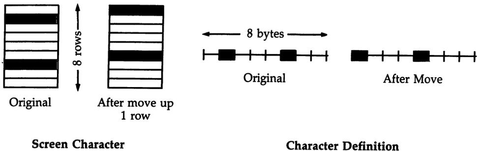
SYS 49152 uses the loop below, which moves only the required portion of the character definitions. (You may need to add a zero byte at the end points.)
