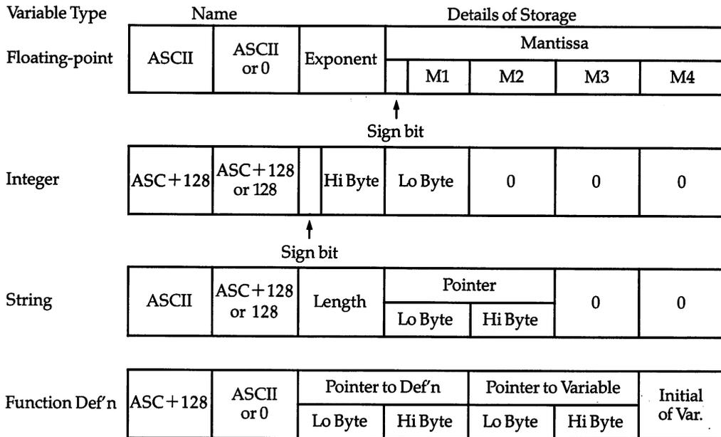
**Floating-point, or real variables (X).** The value is held in five bytes to an accuracy of one part in 2<sup>31</sup> (about two billion).
