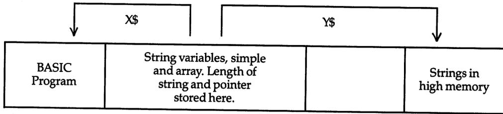
X\$ is stored only in a BASIC program line (for example, 10 X\$="HELLO"). Strings which must be built from other strings are stored in high memory (for example, 20 Y\$=H\$+Z\$).
