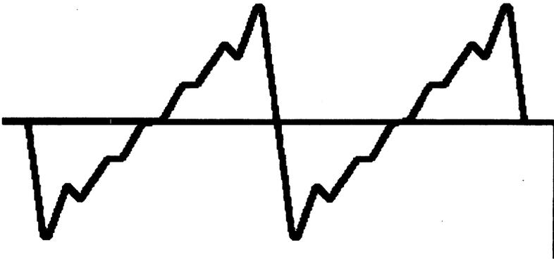
The large numbers of significant harmonics enable this wave to simulate such instruments as the trumpet, oboe, clarinet, and accordion, especially when filtered to change the harmonic balance.
